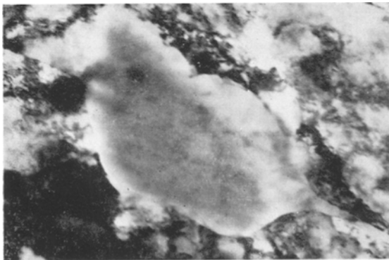
Figure 1 Dislocation-free region seen in a fatigued cold-rolled copper sample (80% red.; S = 7.8 \text{ kg/mm}^2 ; N = 6.8 \times 10^5 ; \times 36\ 000 ).
