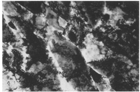
Figure 2 Early form of polygonisation seen in a fatigued cold-rolled copper sample (80% red.; S = 7.8 \text{ kg/mm}^2 ; N = 6.8 \times 10^5 ; \times 18\ 000 ).
